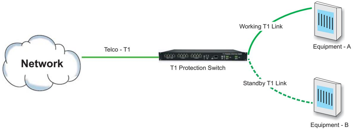
Equipment-A fails - Telco T1 automatically switches to Equipment-B
